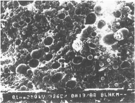
FIGURE 4 SEM micrograph of uncompatibilized PP/SBHN 70/30 blend
